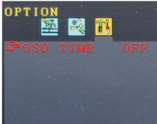
Fig. 13: automatic shutdown deactivated
