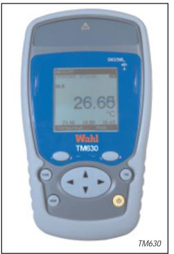
**Statistics** - Maximum, Average, and Minimum are displayed. Reset function allows re-calculating of the values.
