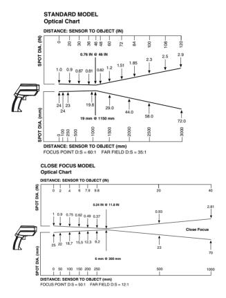
The measured spot size depends on the distance between the object you are measuring and the infrared thermometer.
