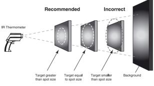
Make sure that the target is larger than the unit's spot size. The smaller the target, the closer you should be to it.
