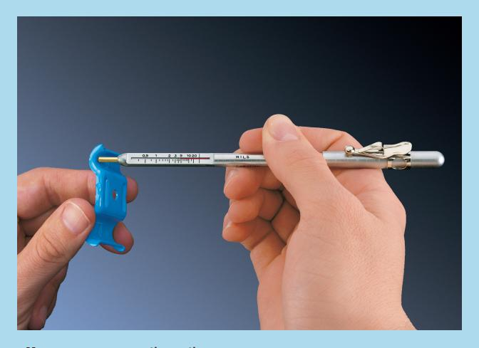
Measures non-magnetic coatings such as paint, enamel, plating, hot-dip galvanizing on steel.
